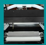
Underside stencil cleaning system with sprinkler. Various combinations of wet / dry and vacuum cleaning are available for cleaning the stencils.
