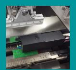
Positioning camera system to teach and recognize the marks of PCB and stencil by up & down camera viewing function.
