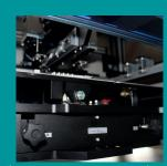
Align the PCB to the template using adjustment screws on the X / Y / R axes
